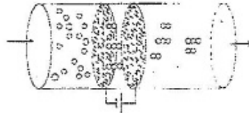
Fig.1 As the fuel flow passes a strong local electric field, the suspended particles aggregate along the field direction, and the viscosity is reduced.
